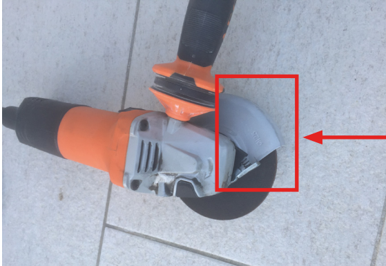
Figure 49. A correctly guarded hand-held cutter/grinder.
