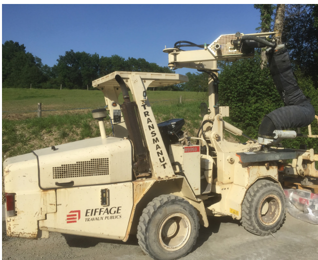
Figures 37 and 38. A vacuum lifter for kerb stone lifting.
