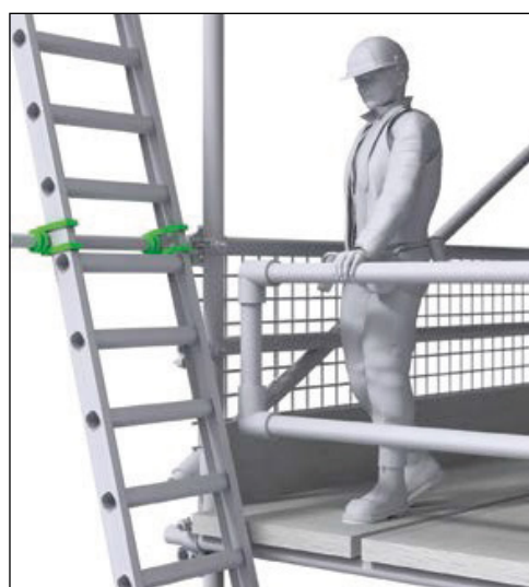
Figure 12. A ladder correctly positioned and secured near the access platform.
