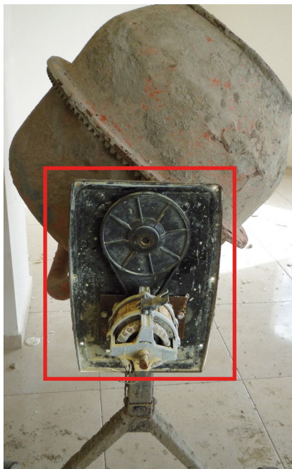
Figure 45. An unguarded drive mechanism on a cement mixer.
