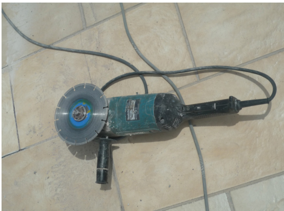
Figure 48. A poorly guarded hand-held cutter/grinder.
