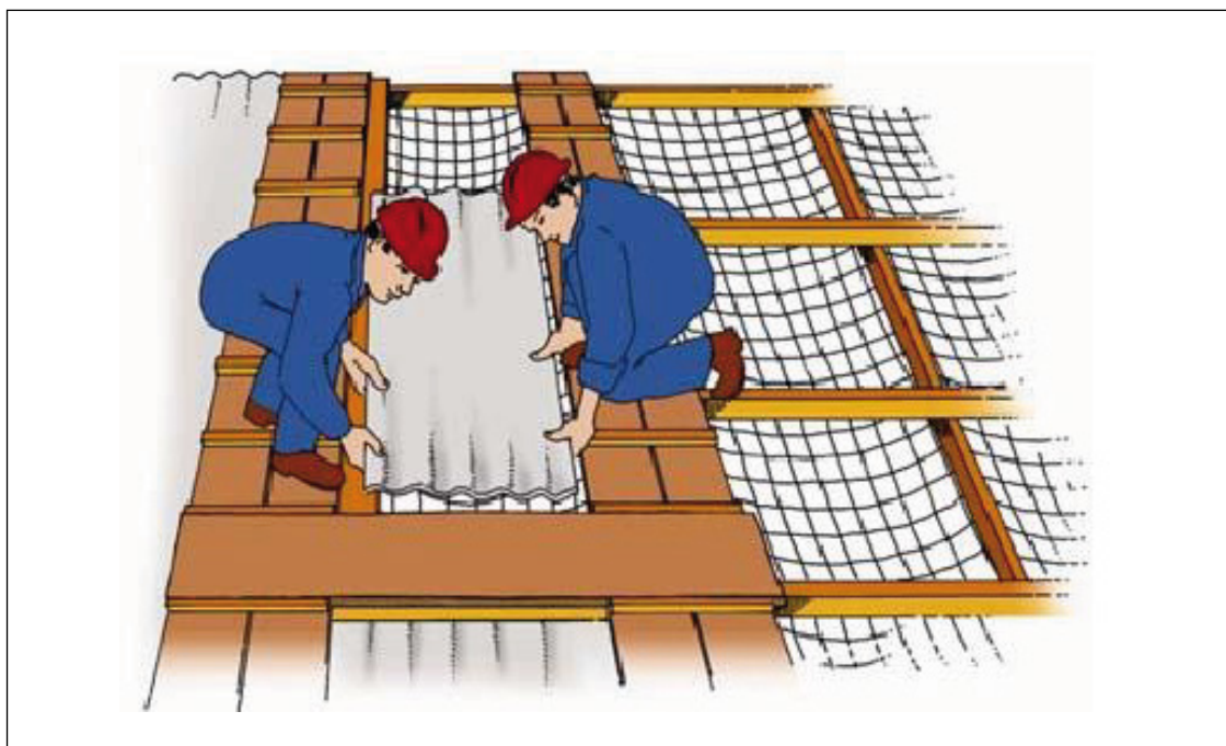
Figure 22. Safety nets in place.
