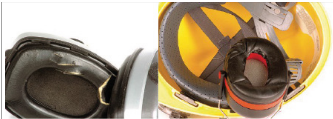
Figures 51 and 52. Hearing protection with split and damaged seals.
