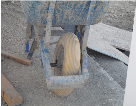
Figure 50. A wheelbarrow with a poorly maintained wheel bearing.
